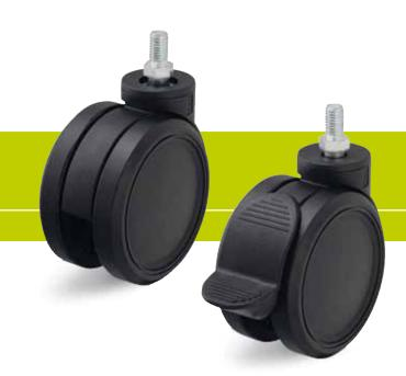
Brackets: LKDB series - Made of high-quality, impactresistant nylon, with high-quality synthetic plain bore in the swivel head, with zinc-plated steel threaded pin, black RAL 9005. Bracket overview: Page 64
